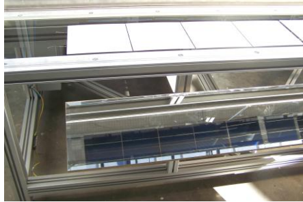
Integrated string inspection
