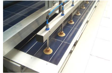
Suction grippers adapt to the modules' height
