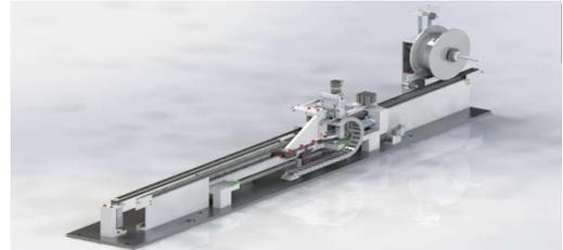
Ribbon handling: stretching, cutting, bending, ...
